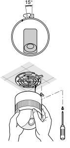
5. Tighten the fixing screw M3 (provided).
