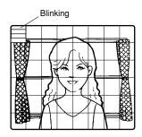
Move the cursor to MASK SET and press the CAM (SET) key. The 48 mask areas appear on the monitor screen. The cursor is blinking in the top left corner of the screen.
