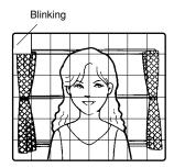
To mask an area where backlight is bright, move the cursor to the area and press the CAM (SET) key. The mask turns white. Repeat this procedure to mask the desired areas.
