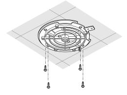
2. Fix the camera mounting base to the ceiling with four screws (not provided, M4).
