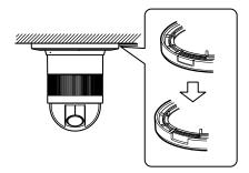
Note: Remove sharp edges to protect the cables.
